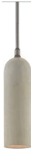
9000-0625 STONEMOSS SLENDER PENDANT H: 16.75" Dia: 3.5" Adjustable: 19.75"h to 57.5"h Canopy: Round, H: 1" Dia: 6" Materials: Wrought Iron/Concrete Finish: Hiroshi Gray/Portland 1 Light Bulb/Socket: B Torpedo Tip/E12
