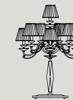
F6+1L Shade 7 E14 x 40W Ø 61 cm - H 82 cm con paralume / with shade
