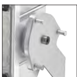
Three-spring hook/release mechanism.
